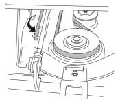
3 Tension the belt with the belt adjuster.
